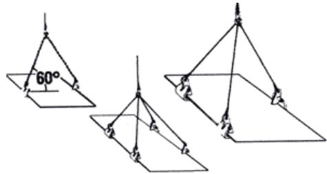
**STEEL PLATES:** Unless otherwise specified, lifting clamps are manufactured to handle hot-rolled steel plates whose Brinell Hardness does not exceed 300. **WARNING: Do not lift plates with coatings or mill scale that prevent the gripping surfaces of the clamp from making positive contact with the base metal.**
