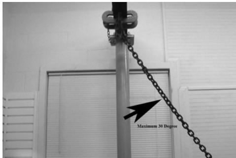
Photograph H. 30 degrees perpendicular to the beam.
